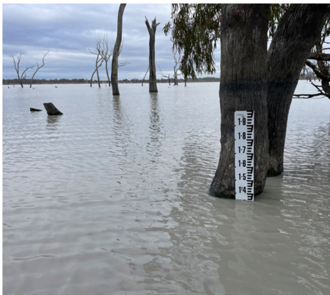
Red Gum Swamp gauge board for surface water monitoring
