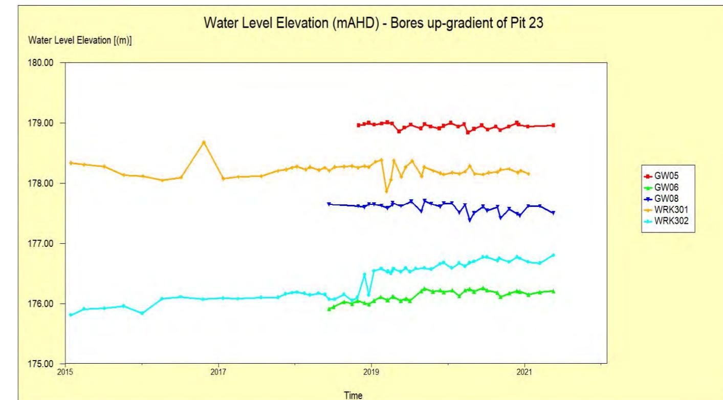
Figure 5: Groundwater elevation (mAHD) – up-gradient bores
