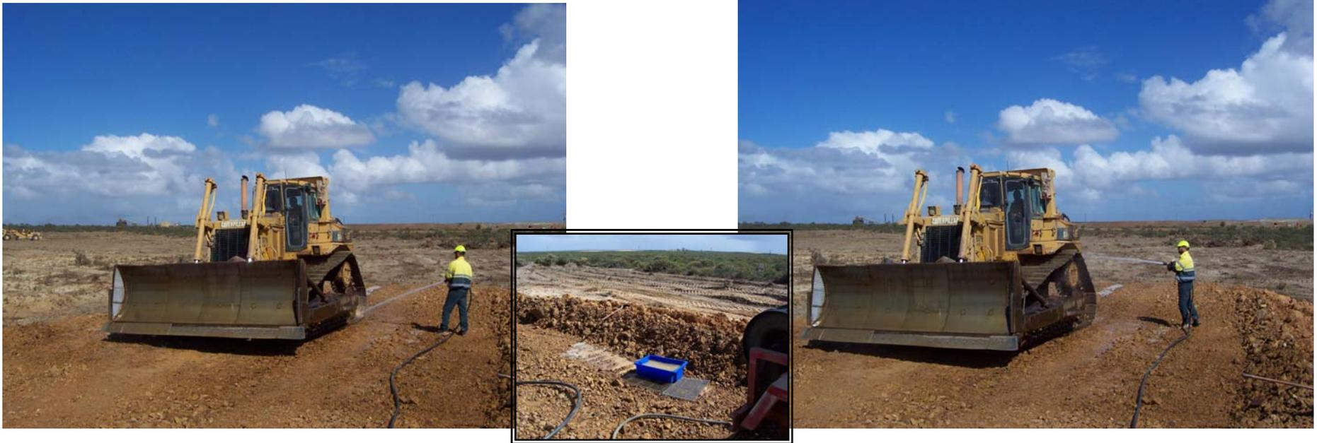
Dozer walked forward to inspect and wash track guides and behind track shoes. Second stage finished off with chlorine wash with dozer walked onto conveyor belt for final inspection (inset; tool and footbath wash-trough with metal separation mats. Dirty wash side to the left of trough with clean side to the right). Final inspection includes inspection under engine canopy, inside operator cabin with floor brushed and pedals inspected for mud etc.
