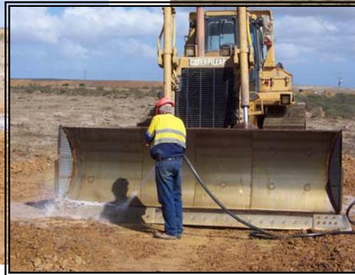
Initial inspection removed all vegetation (sticks, roots, leaves etc) with heavy soil fouling removed with spade-work. Dozer then walked onto first part of ramp for initial stiff brush cleaning and high pressure wash. Photo's show first stage cleaning after dozer walked onto front of ramp.
