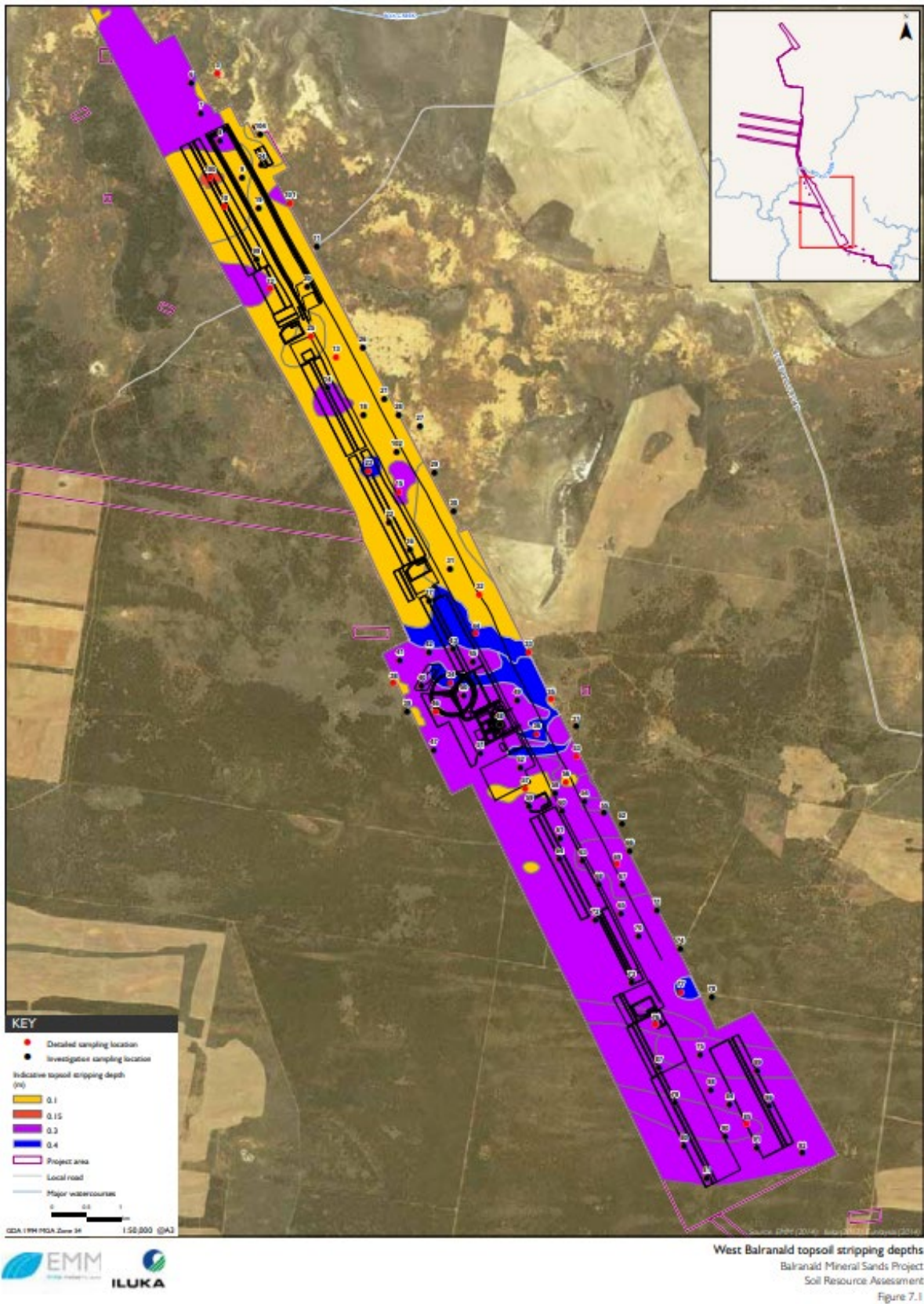
Figure 9 Topsoil stripping depths
